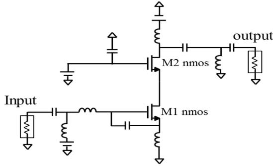
**Figure 2. A Schematic of 2.4GHz cascade single-ended LNA**
