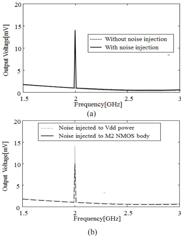
**Figure 8. (a) Noise figure w/o TGV-TGV coupling noise injection and (b) comparison of noise figure between noise injection to Vdd or M2 NMOS body**
