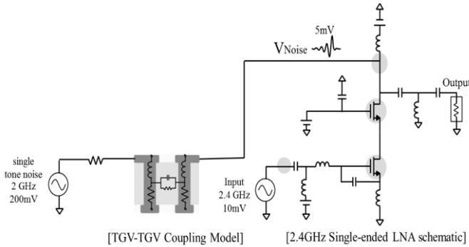
**Figure 5. Simulation setup for noise coupling effects to LNA performance**
