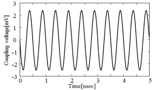
**Figure 6. Time domain waveform of arisen TGV-TGV coupling voltage when 200mV 2GHz single tone noise is injected**
