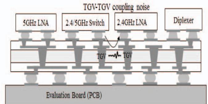
Figure 1. Conceptual figure of TGV – TGV coupling noise effects to LNA on glass interposer
