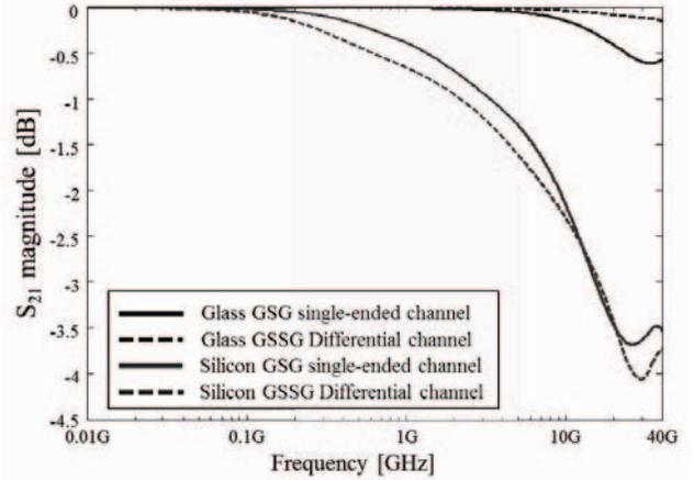
Figure 3.  $S_{21}$  magnitude of single-ended and differential TSV and TGV channel with single via transition
