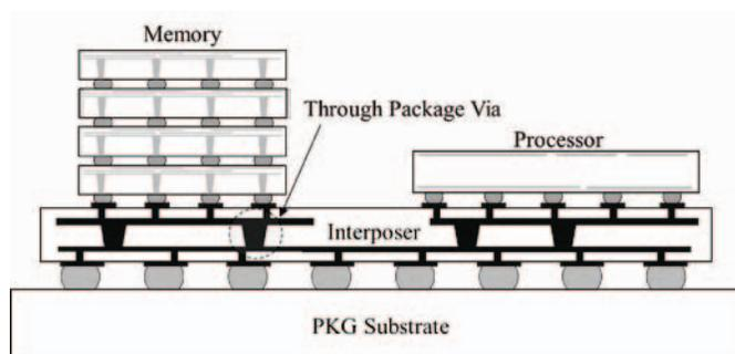
Figure 1. The concept of 2.5D IC with interposer and through package via
