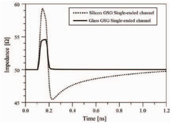
Figure 4. Characteristic impedance of single-ended TSV and TGV channel with single via transition
