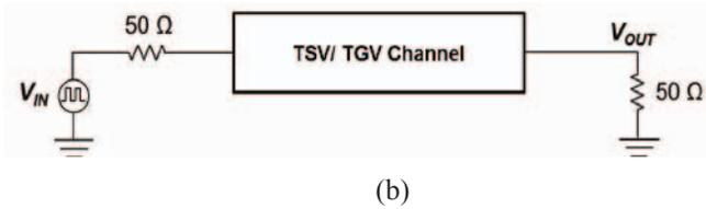
Figure 2. (a) The dimension of TSV and TGV channel for time-domain and frequency-domain simulation (b) Simulation setup for time-domain simulation
