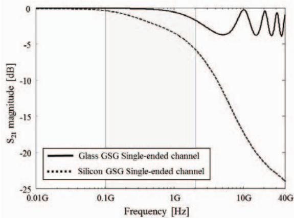
Figure 5.  $S_{21}$  magnitude of single-ended TSV and TGV channel with multiple via transition
