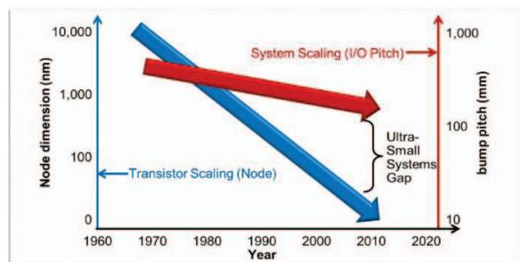
Figure 5: gap between transistor and system scaling for electronics systems
