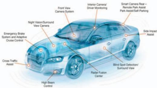
Figure 2: Advanced Driver Assistance Systems (ADAS) application example [6]
