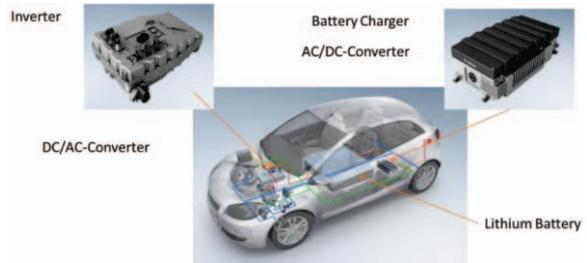
Figure 3: new era in automotive electronics – powertrain of electric vehicles
