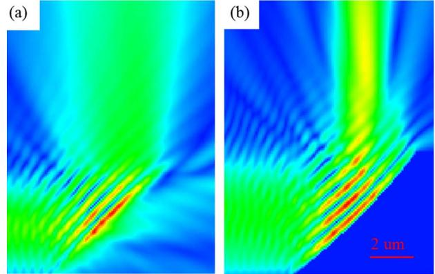
Figure 4. 2D FDTD simulation results for (a) TIR and (b) metallic turning structures with accurately modeled sidewall profile.
