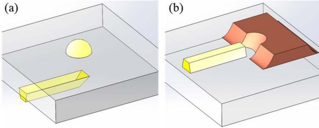
Figure 3. Design of (a) TIR and (b) metallic turning structures.
