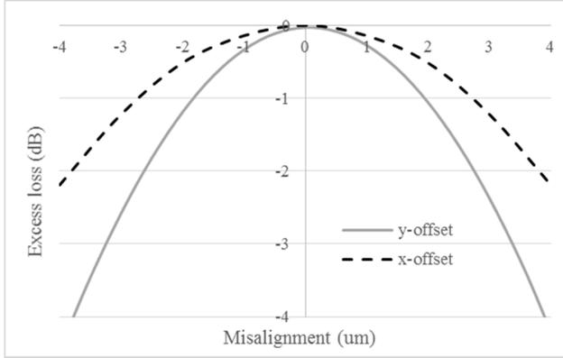
Figure 6. Alignment tolerance of fiber to waveguide interface
