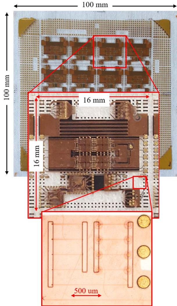
Figure 12. Integrated test vehicle fabricated at panel level, with the TIR turning mirror design implemented at 250  $\mu\text{m}$  pitch.
