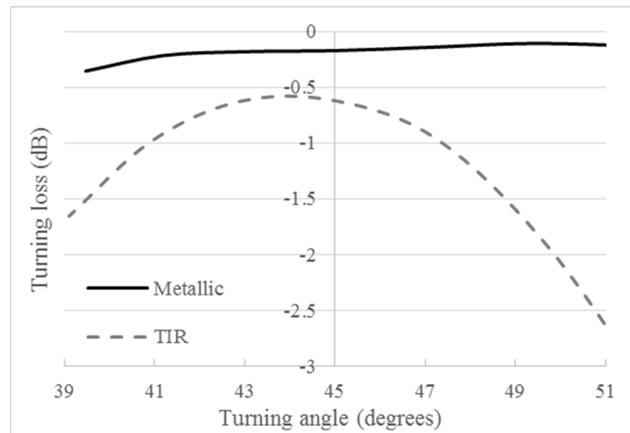
Figure 5. Turning loss sensitivity with respect to turning angle, for both metallic and TIR mirrors.
