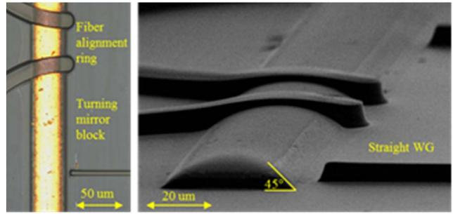
Figure 8. Fabricated metallic coupling structure viewed from top (left) and viewed in SEM.
