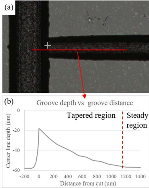
Figure 9. U-groove formation by shallow cut, with extended tapered region.
