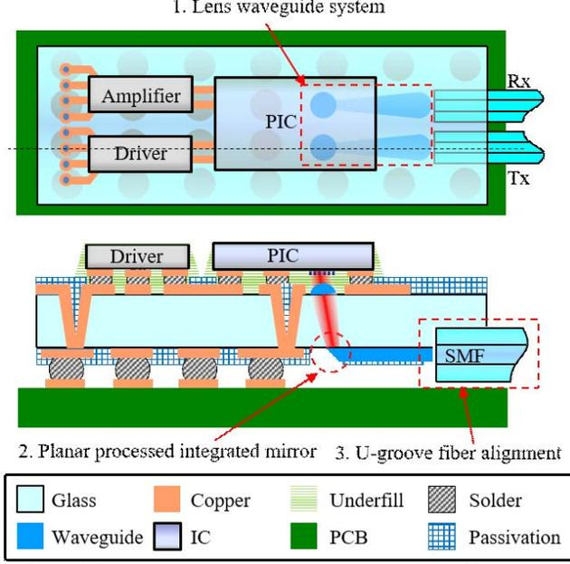
Figure 1. Integration of out-of-plane turning structure and U-groove in glass interposer, for coupling between a gratings based PIC and a SMF.
