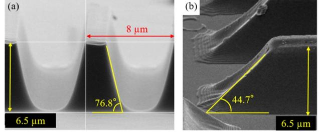
Figure 2. (a) Standard optical waveguide using CYCLOTENE 6505, and (b) planar processed turning mirror using moving mask method.
