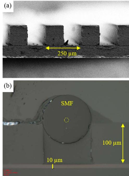
Figure 10. U-groove formation by through slot cut. (a) SEM micrograph of the grooves and (b) cross-section of fiber assembled on one of the grooves.
