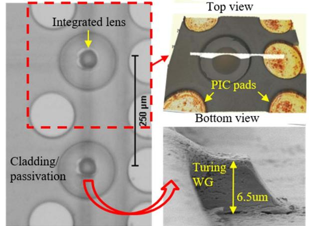
Figure 7. Fabricated TIR coupling structure viewed from top with SEM micrograph of the turning structure at the bottom and confocal micrograph of the lens on top with electrical connections to laser chip.
