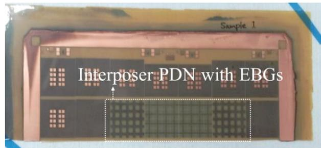
Fig. 5. Glass interposer coupon with EBG patterns are shown in white dotted line.
