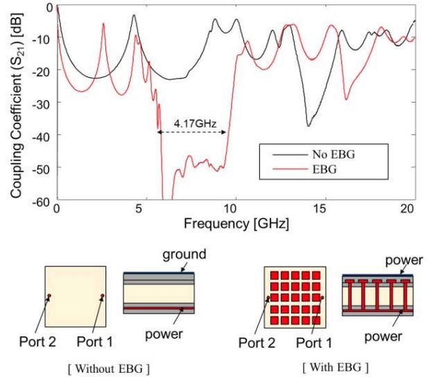
Fig. 10. Measurement of electromagnetic bandgap in the glass interposer PDN with and without mushroom type EBG structures (25 patches)
