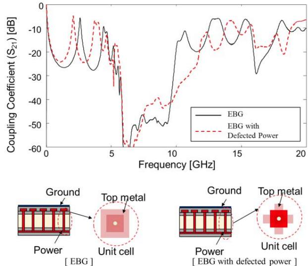
Fig. 11. Measurement of electromagnetic bandgap in the glass interposer PDN with and without defected power in mushroom type EBG structures (25 patches)
