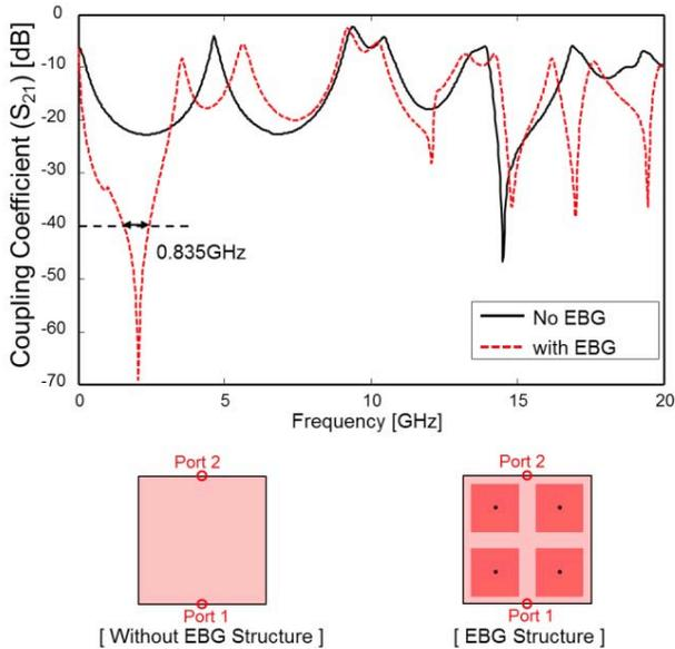
Fig. 6. Noise coupling coefficient with and without EBG (in this case, four additional power patch with 7mm by 7mm in are added in the PDN) is compared. Band-gap is formed around 2GHz and the stop band is 0.835GHz.
