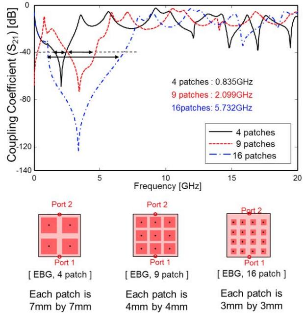
Fig. 8. Impact of altering the number of power patches on electromagnetic bandgap is shown.
