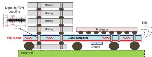
Fig. 1. Noise propagation in the glass interposer PDN is depicted
