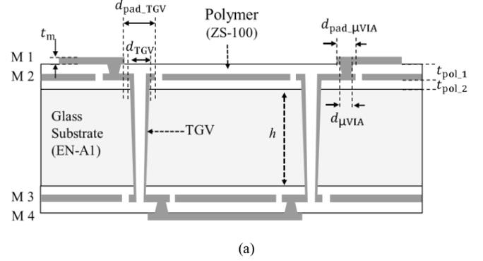
Fig. 2. Cross-sectional view of the glass interposer fabricated. Double sided glass interposer coupons consist of 4 metal layers, glass substrate, polymer, micro-vias and TGVs.
