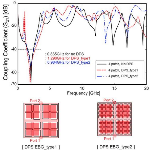
Fig. 9. Impact of defects in the power plane on the electromagnetic band-gap is shown.
