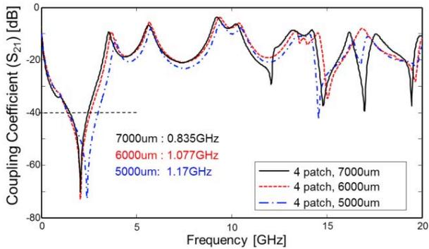
Fig. 7. Effectiveness of altering the size of the power patch on the electromagnetic band-gap was simulated. Changing the dimension did not have great impact on the band-gap's stop-band.
