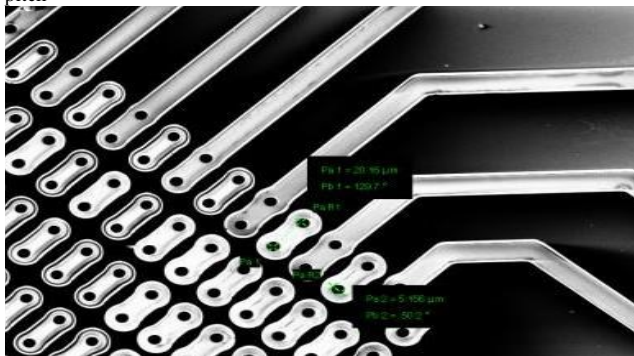
Fig 12. SEM image of the daisy chain structure of 5 \mu\text{m} photovias at 20 \mu\text{m} pitch
