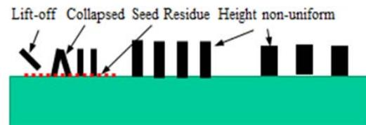
Figure 5. Traces raised on dielectric layer surface with seed layer etching difficulties, plated copper height non-uniform and face trace damages.
