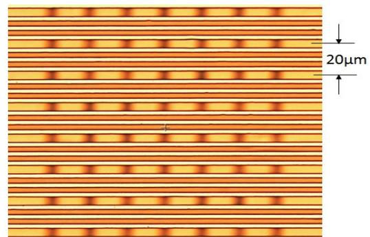
Figure 13. Zoomed in view of embedded fine trenches integrated with small microvias on 100  $\mu\text{m}$  glass. Trench width and space are 3  $\mu\text{m}$  each, microvia diameter is 3  $\mu\text{m}$ , and trench width for via interconnection is 5  $\mu\text{m}$ . The configuration of the new RDL is L/S/Via/T = 3/3/3/5  $\mu\text{m}$ .
