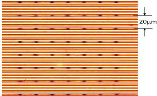
Figure 14. Zoomed in view of embedded fine trenches integrated with small microvias in IF4605 dry film using 100 $\mu\text{m}$  thick glass core. Trench width and space are 2.5 $\mu\text{m}$  each, microvia diameter is 2 $\mu\text{m}$  and trench width for via interconnection is 2.5 $\mu\text{m}$ . The configuration of the RDL is L/S/Via/T = 2.5/2.5/2/2.5  $\mu\text{m}$
