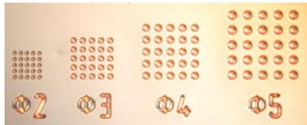
Figure 7. Micrograph of 2 to 5 $\mu\text{m}$  microvias formed in 5  $\mu\text{m}$  thick photosensitive dry film IF4605. The minimum via diameter opened was 2  $\mu\text{m}$  at 4  $\mu\text{m}$  pitch
