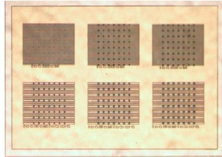
Figure 12. Fabricated test coupon with 6 structures consisting of embedded fine trenches integrated with small microvias on 100  $\mu\text{m}$  thick glass core with good alignment; via pitch for all is 20  $\mu\text{m}$ , min. via is 2  $\mu\text{m}$ .
