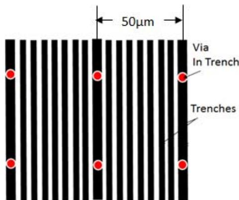
Figure 2. New type RDL via-in-trench routing configuration on panel glass by Photo Embedded Trench approach with about 10X increment of wiring capability compared to figure 1.
