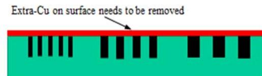
Figure 6. Embedded trenches: traces buried in dielectric layer and protected. Surface flat, no seed layer etching required. Extra copper on surface removing is needed.
