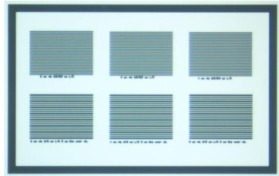
Figure 8. Via-in-line test coupon for exploring routing capability of embedded photo trenches and photovias. The line and space for top 3 structures is 2.5  $\mu\text{m}$  and for bottom 3 structures is 3  $\mu\text{m}$ .
