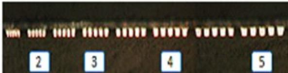
Figure 10. Cross-sections of embedded 1.5 to 5  $\mu\text{m}$  copper traces in PN-0371D dielectric after surface copper etching and completed embedded traces with flat copper surface. The height of the traces is 4.8  $\mu\text{m}$  and thus the trench aspect ratio is 3.2
