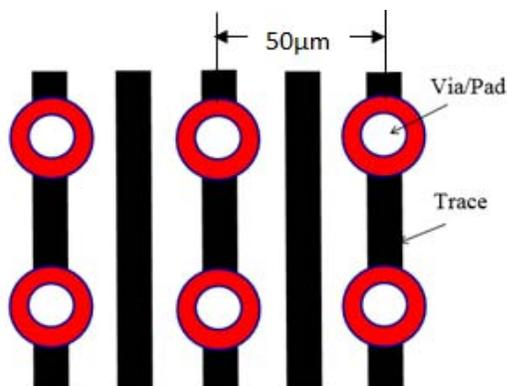
Figure 1. Typical fine pitch RDL via-in-pad routing configuration on panel organic interposer by SAP with one wire in a 50um pitch
