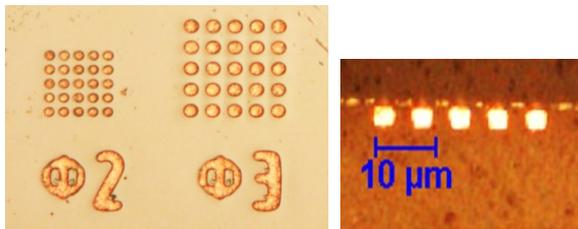
Figure 11. Top view of 2 and 3  $\mu\text{m}$  vias after Cu plating and surface copper etching (left) and cross section of a row of 3  $\mu\text{m}$  vias (right).
