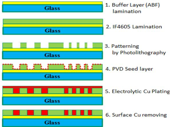
Figure 9. Photo Trench (or Photo Via) Fabrication process steps.
