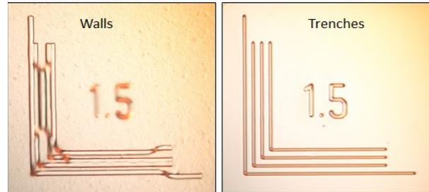
Figure 4.  $1.5\ \mu\text{m}$  wide raised structure (wall) collapsed (left),  $1.5\ \mu\text{m}$  embedded trenches stable (right).
