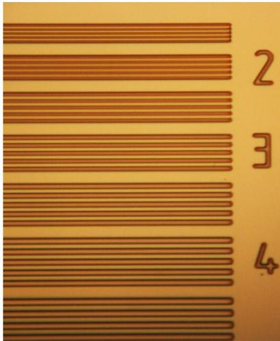
Figure 3. Micrograph of  $1.5$  to  $4.5\ \mu\text{m}$  comb structure photo trenches fabricated on thin glass panel using  $\sim 5\ \mu\text{m}$  thick liquid polymer dielectric PN-0371D film
