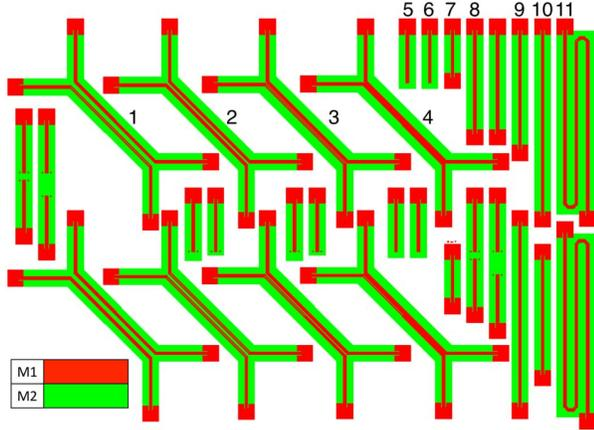
Figure 4. High-speed electrical design test structures on two-metal layer glass interposer test vehicle (TPV at differential signal launch).
