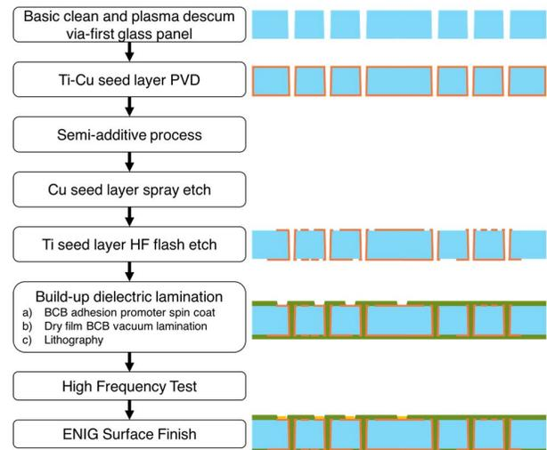
Figure 6. Panel-based process flow to fabricate RDL on bare glass.
