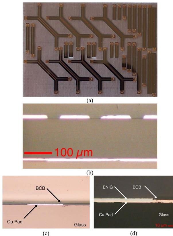
Figure 7. Glass panel fabrication results including: (a) crosstalk test structure overview, (b) differential pair cross section before passivation and cross section details (c) before and (d) after surface finish.
