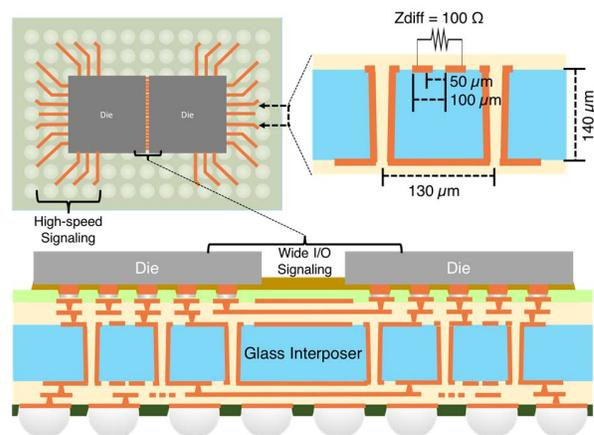
Figure 1. 2.5D glass interposer cross section schematic with top view showing high-speed and wide I/O signal regimes with a detailed cross section of the high-speed interconnect layer.
