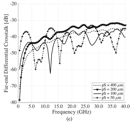
Figure 5. 3D electromagnetic simulation of RDL on glass (a) model for crosstalk, (b) near-end differential crosstalk, and (c) far-end differential crosstalk for pair spacing  $pS = 50 \mu\text{m} - 400 \mu\text{m}$ .
