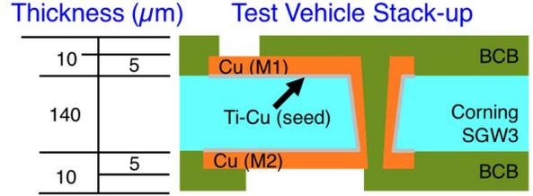
Figure 2. High-speed electrical test vehicle stack-up.
