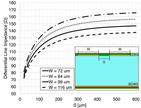
Figure 3. 2D electromagnetic differential line impedance simulation of high-speed RDL on bare glass.
