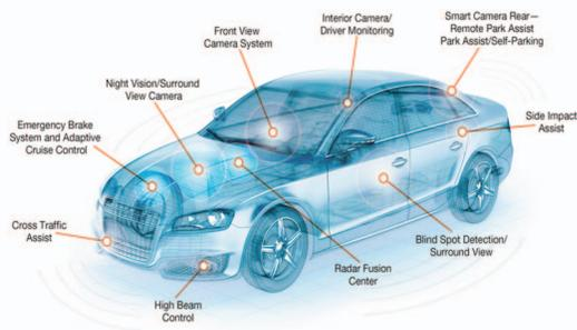
**Figure 2:** Advanced Driver Assistance Systems (ADAS) application example [6]
