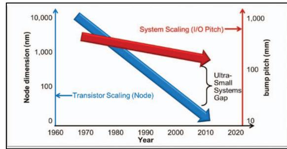
**Figure 5:** Gap between transistor and system scaling for electronics systems
