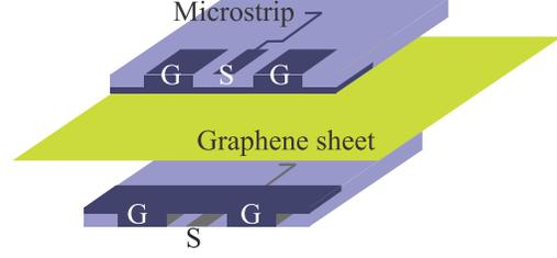
Figure 2. Characterization setup with microstrip structures for the shielding effectiveness (SE) measurement of graphene sheets. The signal pads (S) are placed between two ground pads (G).
