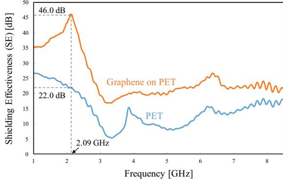
Figure 3. Shielding effectiveness measurement of graphene shields.
