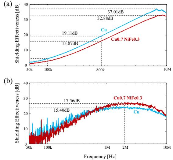
Figure 6. Shielding effectiveness measurement of Cu, NiFe, and multi-layered structures.
