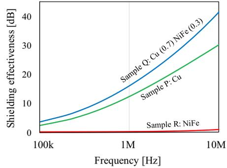
Figure 4. Shielding effectiveness simulation of metal, ferromagnetic, and multi-layered samples.
