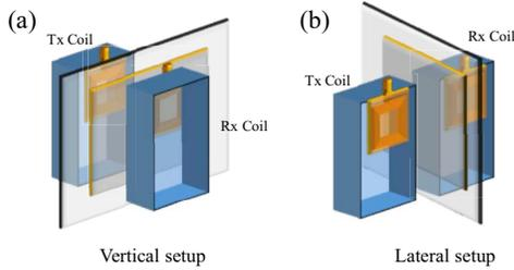
Figure 5. Characterization setups to measure the  $S_{21}$  parameter of (a) vertical and (b) lateral noise coupling.
