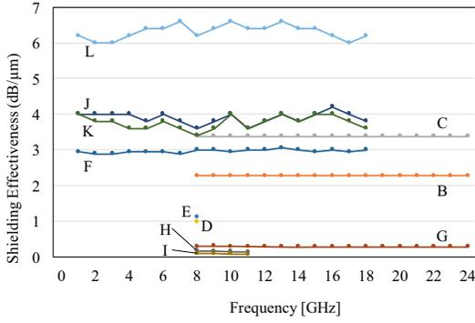
Figure 1. Shielding effectiveness comparison of Samples B-M.
