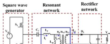
Figure 3. Schematic diagram of LLC resonant converter topology
