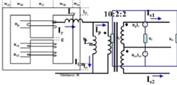
of the core should guarantee that the flux density value is lower than the maximum saturation value of the magnetic core material.
