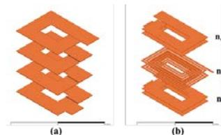
Figure 7. Winding configurations for discrete components (a) resonant inductor and (b) transformer.
