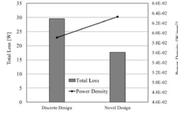
lower overall loss with a 7% increase in power density. The total core volume of discrete planar magnetics itself is smaller than the novel core design, but the overall volume of the two components, including the winding dimensions, exceeds the volume of the novel design. Another notable advantage of the novel design is the low core profile of less
