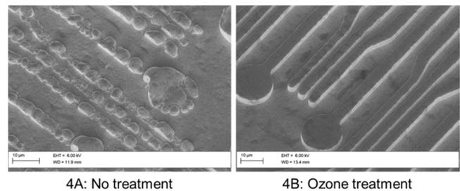
Fig. 4. SEM (10  $\mu\text{m}$  scale) comparison of fine line RDL after copper electroplating on substrates with no treatment (4A) and ozone treatment (4B).
