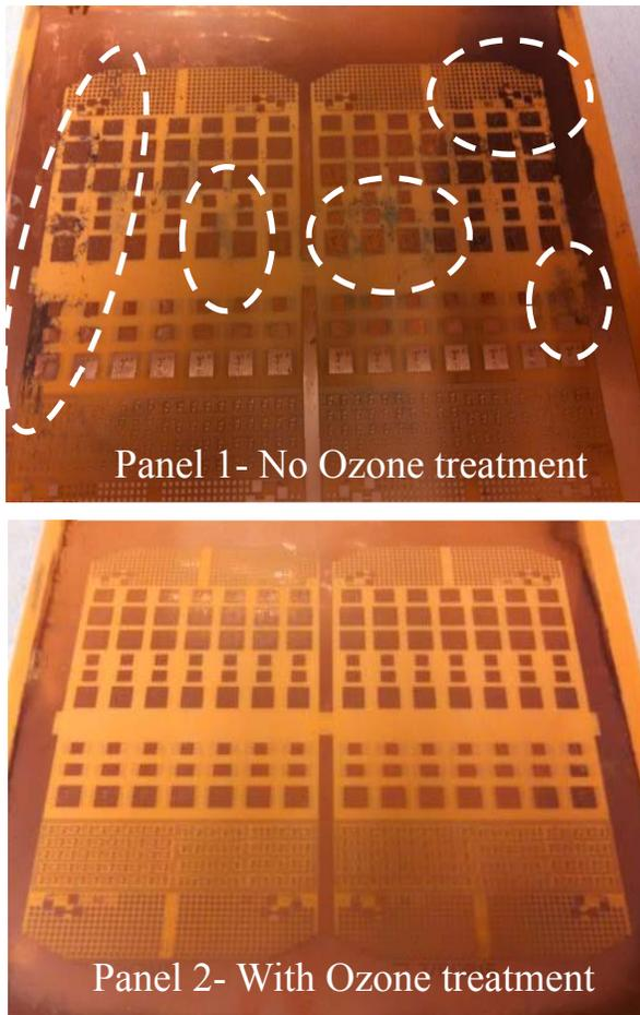
Fig. 7. Comparison of panels processed without (panel 1) and with additional ozone treatment step after DFR strip to highlight the effective removal of DFR residue from the panel using ozone treatment post DFR strip. Defective regions on panel1 are highlighted within the dashed ovals.
