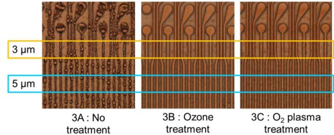
Fig. 3. Comparison of fine line RDL features after copper electroplating on substrates with No Treatment (3A), ozone treatment (3B), and O<sub>2</sub> plasma treatments (3C) illustrating the improvement in plated line quality resulting from wettability improvements of the surfaces with plasma or Ozone treatments.
