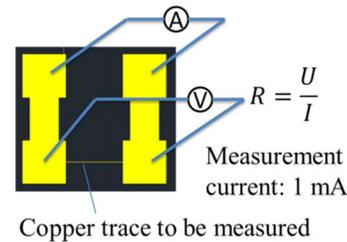
Fig. 6. Structures used for measuring line resistance and RDL yields, 2mm long traces were measured (with 5 μm and 8 μm widths) to quantify the yields. Note picture is not to scale.
