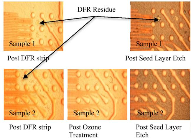
Fig. 8. Removal of DFR residue after strip using Ozone treatment of a panel with RDL illustrating the complete removal of DFR residue with the ozone treatment leading to yielded panel with no residual seed layer. Note the removal of DFR residue from the seed layer surface after the ozone treatment on sample 2. Untreated DFR residue (sample1) result in partial removal of seed layer causing losses in panel yields
