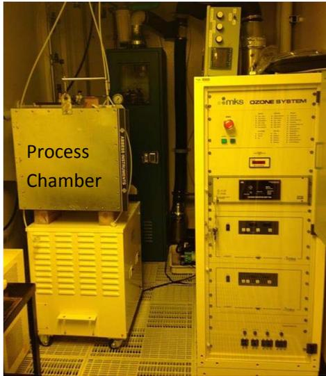
Fig. 2. Setup of the ozone treatment system at PRC. The ozone delivery system is on the right while the “box” chamber is shown on the left. The exhaust from the chamber is routed to an ozone destruct (not shown) to convert any unused ozone to oxygen.
