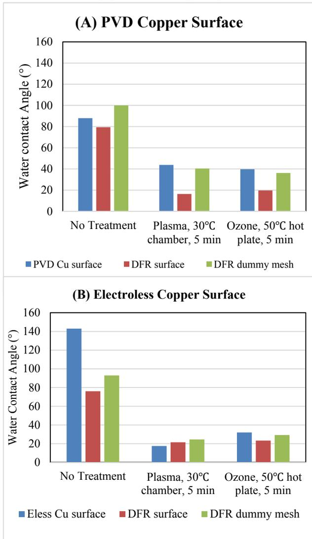
Fig. 5. Comparison of water contact angle (wettability) of the various regions on the panel surface on substrates with No treatment, O<sub>2</sub> plasma treatment or ozone treatments on two types of Cu Seed layers deposited using PVD (A) or electroless Cu (B). Both plasma and ozone treatments are effective in significantly reducing the water contact angle across different regions of the panel.
