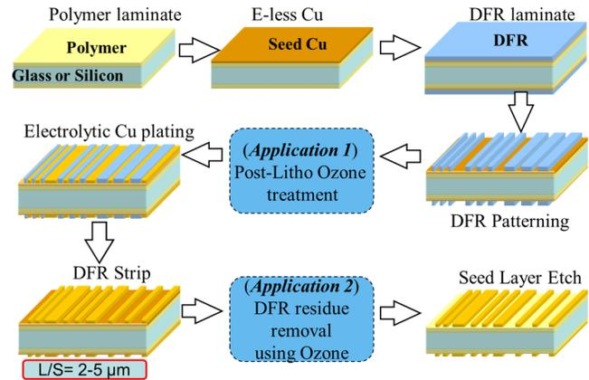
Fig. 1. Two potential applications of ozone treatments evaluated in a semi-additive process for RDL fabrication.
