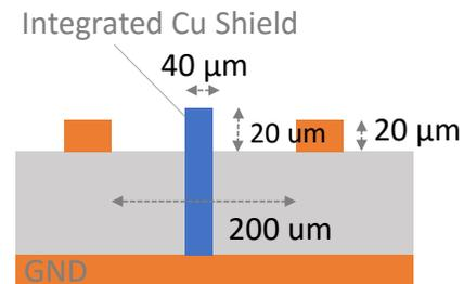
Figure 4. 3D view of the trench-based shield extending above the plane of the signal lines.
