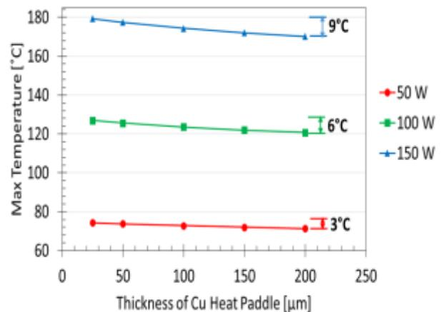
Fig 8. Maximum temperature plotted against the heat paddle thicknesses, (25, 50, 100, 150, 200  $\mu$ m) for each power applied (50, 100, 150W), and showing the change in temperature between 25, and 200  $\mu$ m for each power level.
