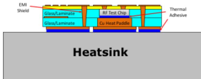
Figure 1. Laminate (LFO) or Glass Fanout (GFO) with Integrated Heat Spreaders and EMI Shields
