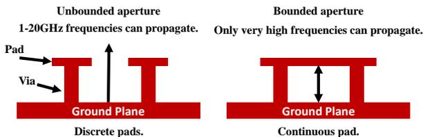
Figure 3. Lateral view of via-array shields to compare the aperture for different scenarios.
