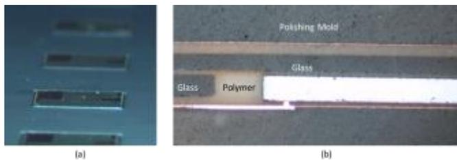
Figure 11. (a) Top View and (b) Cross-section of Glass Fanout (GFO) package.
