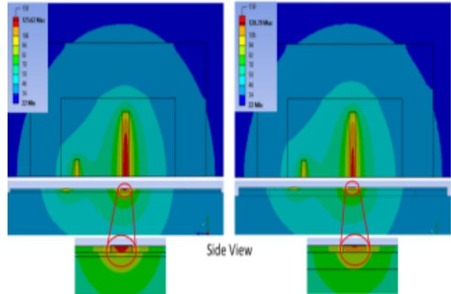
Fig 7. Temperature distribution for the 50 (Left) and 200  $\mu$ m (Right) Cu heat paddles at 100 W.
