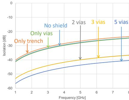
Figure 2. Comparison of TL-TL coupling in presence of trenches and different via-arrays configurations.
