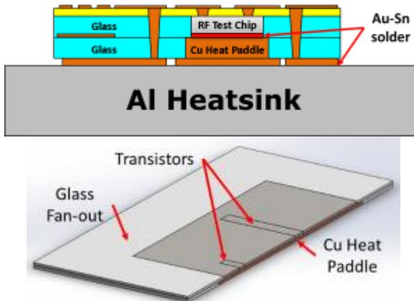
Fig 6. Thermal stack and test package used to model thermal performance.
