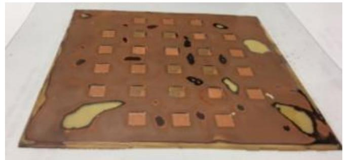
Figure 9. Laminate fanout (LFO) panel with embedded die on copper heat spreaders in selected sites, showing warpage induced planarization challenges.
