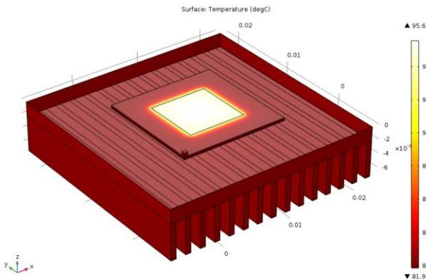
Figure 5 Result of Design with Array of Fins on Heat Sink to Facilitate Convection at 65°C Ambient Temperature with Maximum Temperature of 95.6°C
