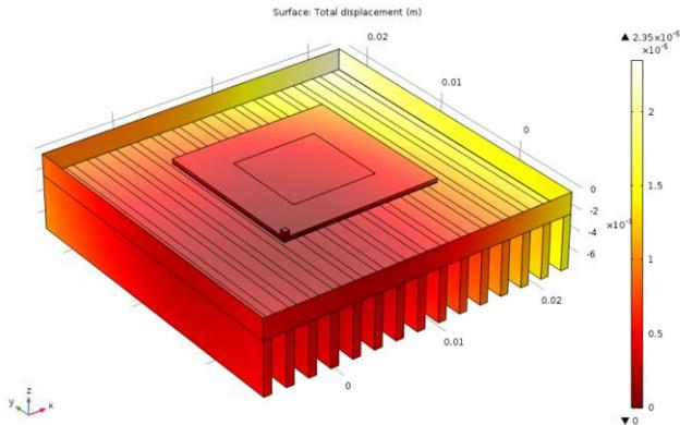
Figure 8 Deformations from Solid Mechanics Stress Simulation for 65°C Ambient Temperature
