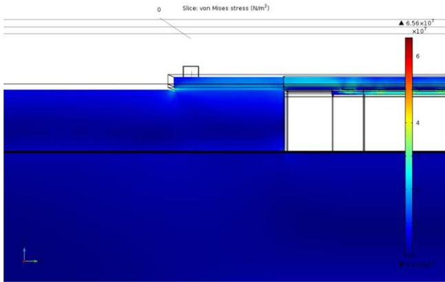
Figure 7 von Mises Stresses from Solid Mechanics Stress Simulation for Temperature Distribution Shown in Figure 5
