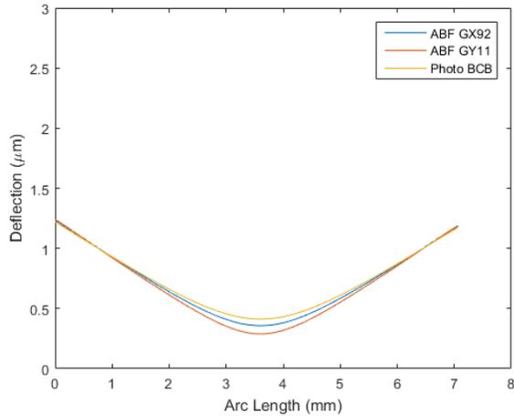
Figure 9 Solid Mechanics Deformation Simulation with 3 Layers of Glass with Middle Cavity Layer and Polymer Between Each Layer as Function of Distance along the Diagonal on the Top Surface with Bonding Temperature of 105°C
