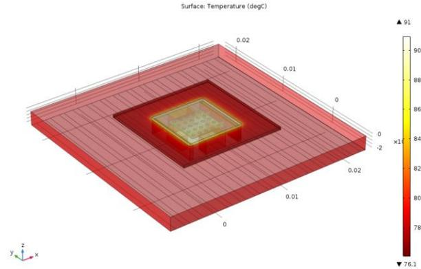
Figure 3 Results of Initial Model Tested at 20°C Ambient Temperature with Maximum Temperature of 91°C
