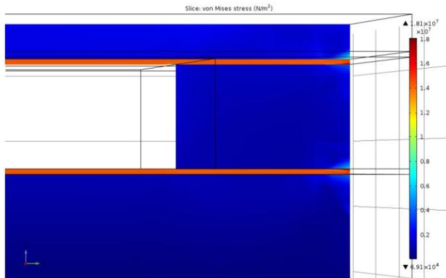
Figure 10 von Mises Stresses for a Partial Slice of Photo BCB Polymer Stress Simulation at Room Temperature After Bonding at 105°C
