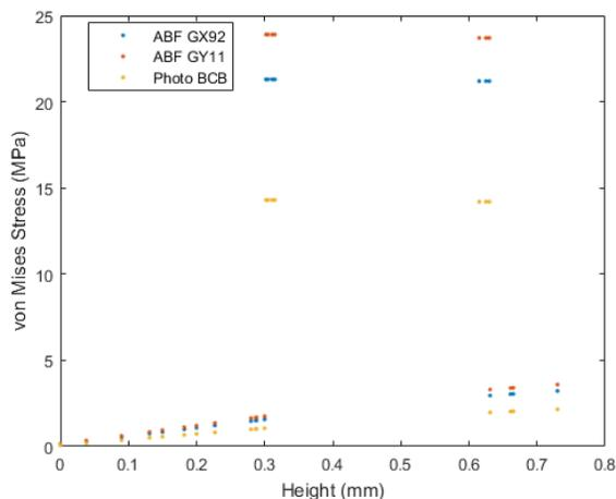
Figure 11 Stress in the Midpoint of the Bonding Structure as a function of Height at Room Temperature After Bonding at 105°C
