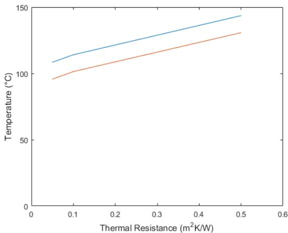
Figure 6 Compilation of Several Models Run with Varying Thermal Contact Resistance with Contact Area Between Substrate
