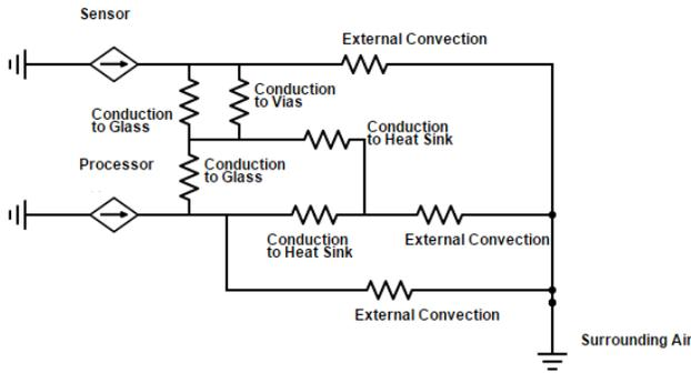
Figure 1 Thermal Circuit Model of Lumped System
