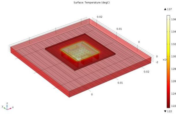
Figure 4 Results of Initial Model Tested at 65°C Ambient Temperature with Maximum Temperature of 137°C
