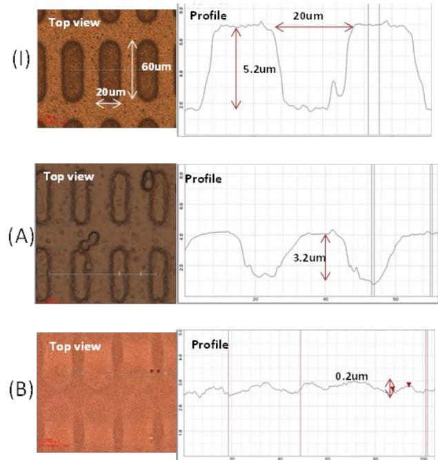
Figure 7. Trench filling by different electrolytic plating processes. (I): before plating, (A): after 40 min plating at 10 A with tank A, (B): after 40 min plating at 10 A with tank B
