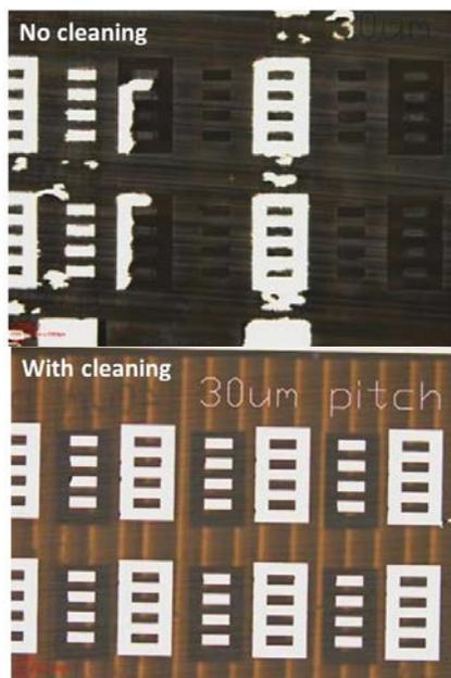
Figure 9. Trench structures after surface planarization process. Sample without desmear cleaning (top) and with desmear cleaning (bottom)
