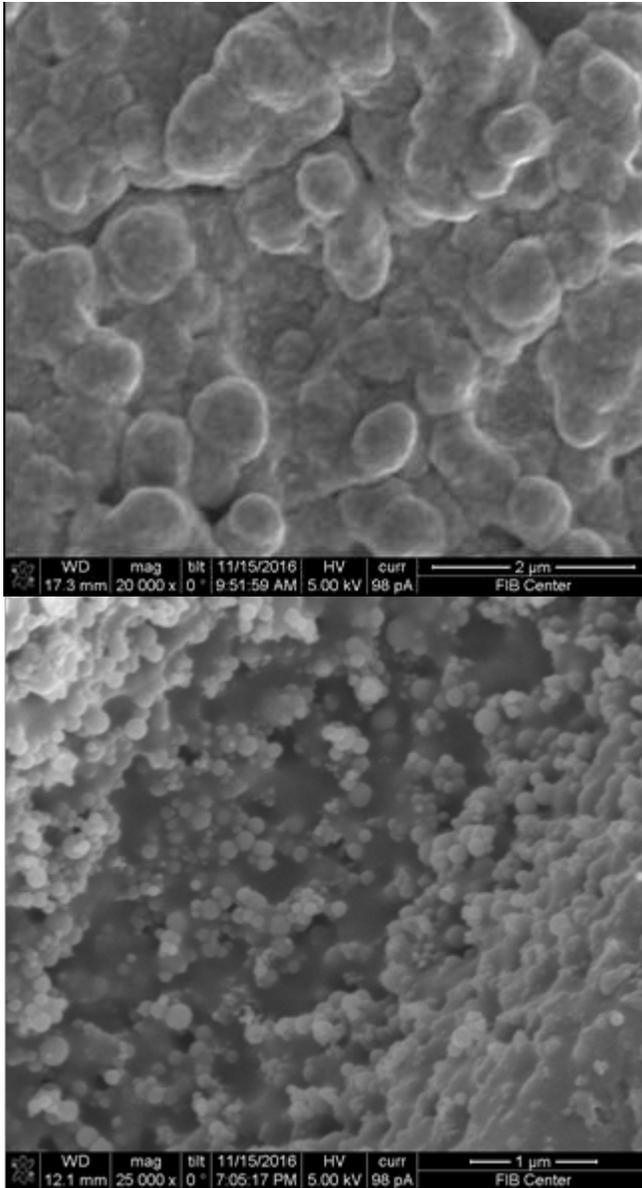
Figure 3. SEM images of filler particles in GX92 (top) and GY50 (bottom)
