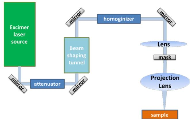
Figure 2. Beam delivery system schematic for excimer laser ablation
