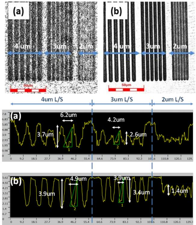
Figure 4. Top view (upper) and line profile (lower) of 2, 3 and 4  $\mu\text{m}$  line and space trenches in GX92 (a) and GY50 (b)
