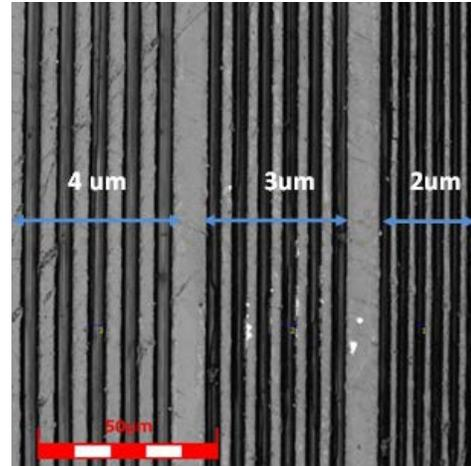
Figure 5. Top view of the 2 – 4  $\mu\text{m}$  ablated trench in polyimide
