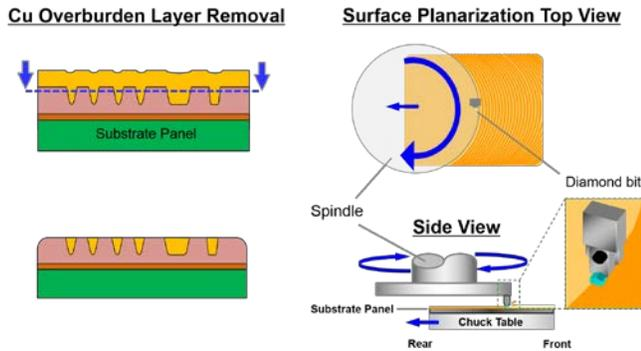
Figure 8. Illustration of Cu overburden removal by a surface planarization process
