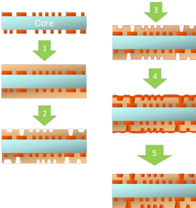
Figure 1. Process schematic of embedded trench processes
