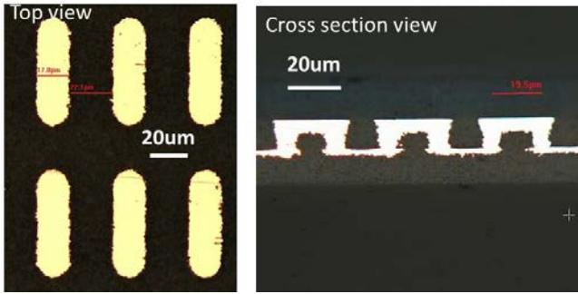
Figure 11. Top view (left) and cross section view of the daisy-chain structure with 20  $\mu\text{m}$  via pitch by embedded trace processes
