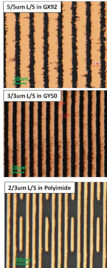
Figure 10. Fine pitch trenches formed in GX92 (top), GY50 (middle), and polyimide (bottom)
