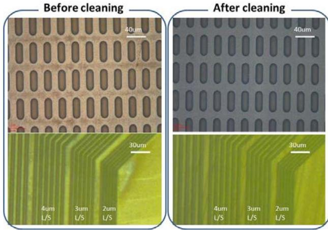
Figure 6. Removal of surface debris by 3min chemical desmear of laser trenches without damaging fine trenches
